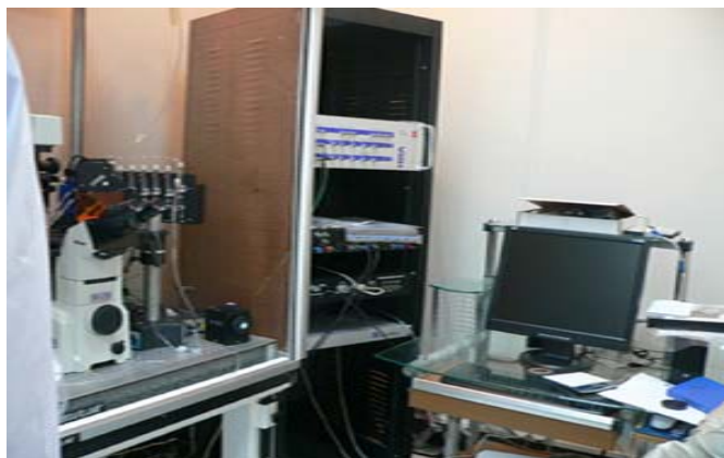
Fig. 2: Patch-clamp technique set-up to record the electrical parameters.
